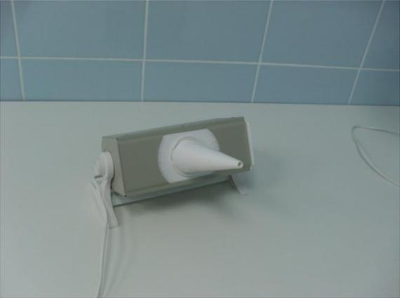
A small, rectangular ultraviolet irradiator with a white nozzle-like protrusion on the front. It is connected to a power cord.                                                |
